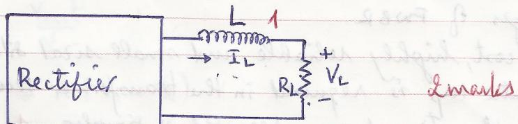
(iii) choke input filter : LC filter 1
